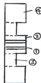
$$m_1 = 8800 \cdot \left[ \frac{\pi}{4} (0.016^2 - 0.012^2) \cdot 0.014 \right] = 0.0108372 \text{ kg}, \quad \bar{x}_1 = 7 \text{ mm}$$
